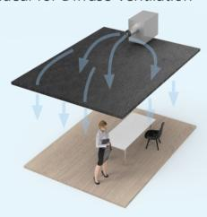
Diffuse ventilation is a method where the ventilation system blows fresh air over a suspended ceiling, which then seeps down through the ceiling's open surfaces. The ceiling consists, for example, of a wood/aluminum frame mounted with FiberAcoustic® sound fabric. This process creates a slight overpressure, ensuring silent and draft-free airflow in the room.
