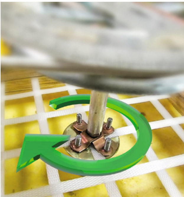
Figure 13 Application of torsional stress to Secugrid® geogrid sample
