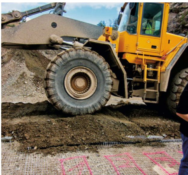
Figure 15 Installation damage factor ( RF_{10} / A_2 ) determined by a field trial in a quarry
