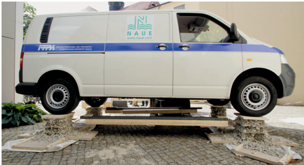
Figure 2 Secugrid® geogrid reinforced stone columns carry a nearly 2 ton heavy delivery van during a live experiment (see http://www.naue.com/en/naue-tv/geogrid-experiment.html )
